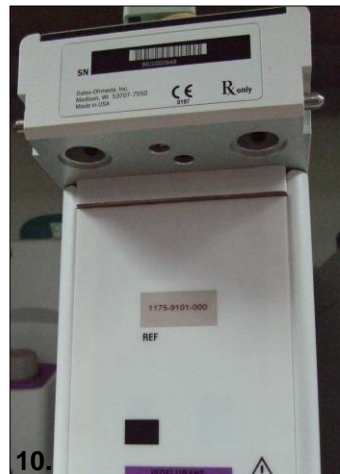
Tec 7 Ohmeda Back, -Looks like back of Tec 4, & 5 (Ohmeda Mount Compatibility Block)
